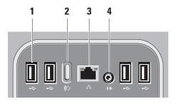
1 USB 2.0 connectors (4) — Connects to USB devices, such as a mouse, keyboard, printer, external drive, or MP3 player. Wireless sync button — Reestablishes the connection between
